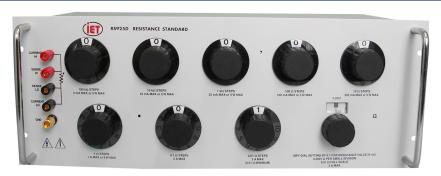
The IET (esi) RS925D is a four-terminal, continuously variable decade resistor for the most exacting calibration and test applications.
