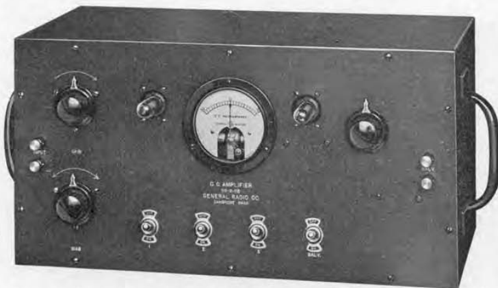
FIGURE 1. A two-stage direct-current amplifier, a piece of special equipment built by the General Radio Company
