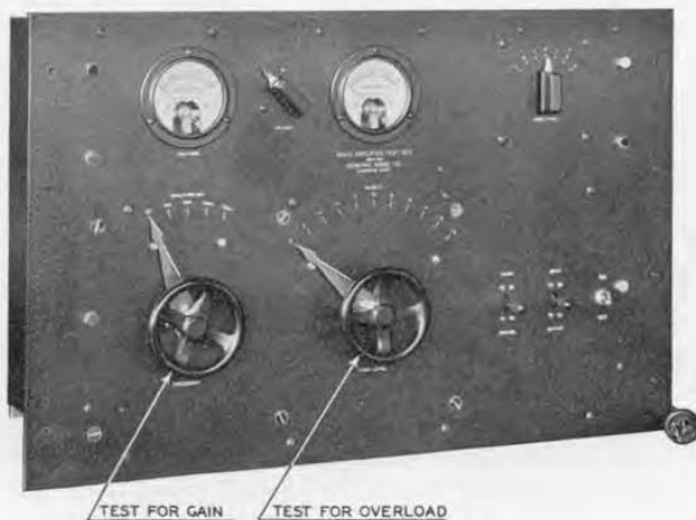
FIGURE 3. The audio-amplifier test set as built by the General Radio Company for the Victor Talking Machine Company
