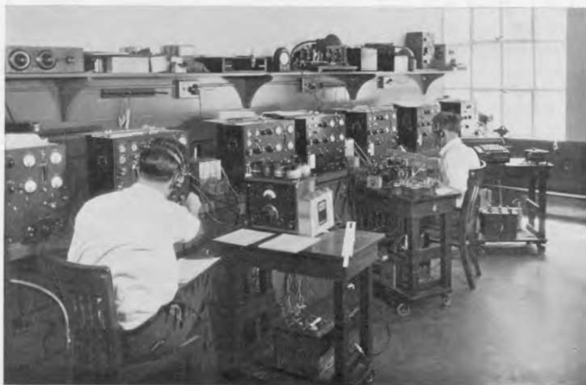
Calibrating a group of special self-checking heterodyne wavemeters designed and built by General Radio for the United States Coast Guard
