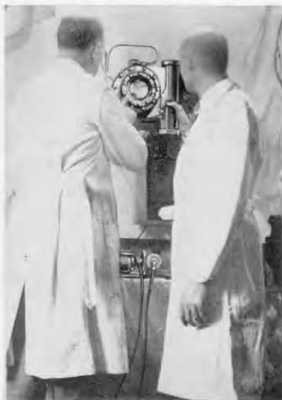
Norge engineers viewing the operation of the Rollator by means of the Edgerton Stroboscope
