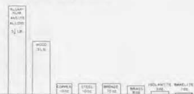
FIGURE 2. Approximate proportions of materials used in a TYPE 722-F Precision Condenser
