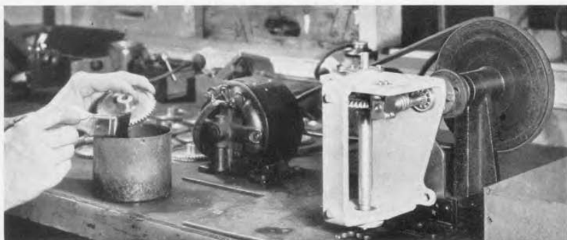
FIGURE 4. At the right is shown the motor-driven assembly for "wearing-in" the worm and gear. After this is finished, the gears must be washed in gasoline, as shown at the left, to remove the fine particles of grinding compound.
