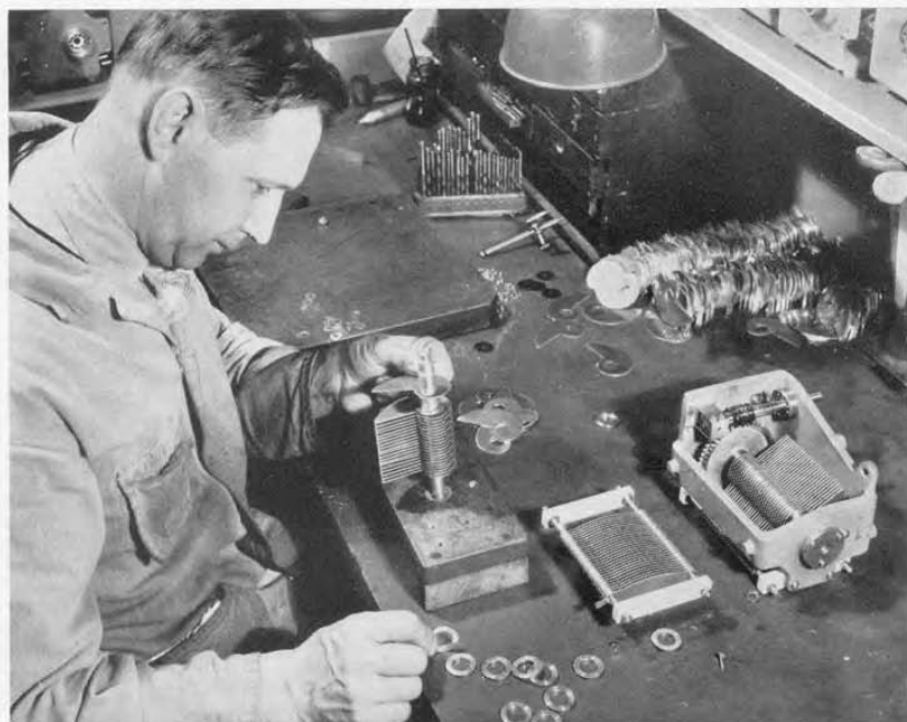
FIGURE 5. Assembling the rotor plates on the shaft. At the right may be seen a stator assembly and a completed condenser
