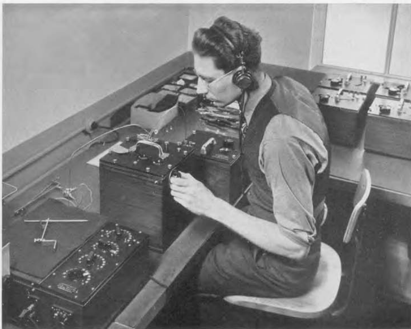
FIGURE 3. Calibrating a TYPE 722-F Precision Condenser
