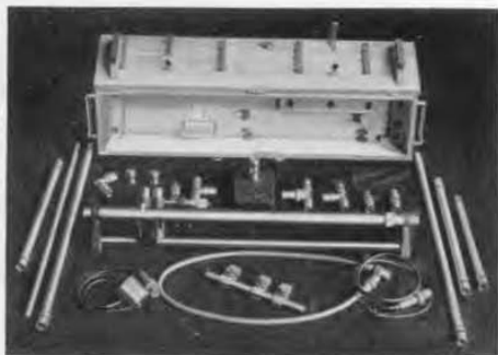
Figure 1. View of the storage box, showing the various coaxial elements that are accommodated.
