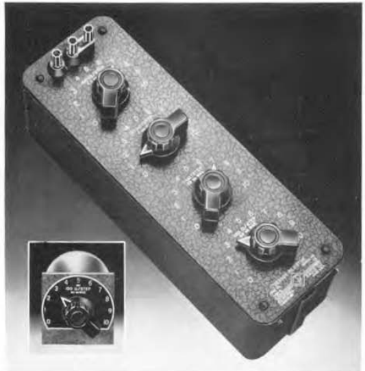
Figure 1. View of a Type 1432-A Decade Resistor. Inset at lower left shows Type 510-D Decade-Resistance Unit.
