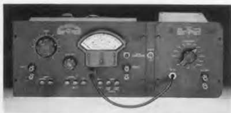
Figure 5. View of the Type 1231-PSR Filter arranged for relay-rack mounting with the Type 1231-B Amplifier and Null Detector. The filter panel attaches to the amplifier panel to make the assembly the correct width for mounting in a 19-inch relay rack. The narrow strip between the two panels carries a switch for the a-c power supply that is optional with the amplifier.
