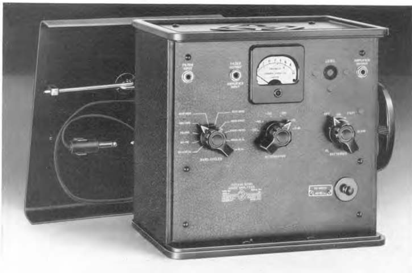
Figure 1. View of the Type 1550-A Octave-Band Noise Analyzer with cover removed to show panel.
