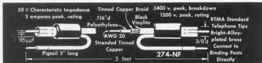
Figure 13. Dimensional sketches, with specifications, of the Type 274-NF Shielded Lead Assembly.
