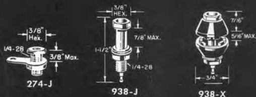
Figure 9. Dimensional sketches of the three standard General Radio jack terminals for banana plugs.
