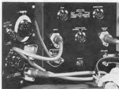
Figure 10. View showing connections to the Type 1001-A Standard-Signal Generator and the Type 1023-A Amplitude Modulator using Type 874 Coaxial Connector. Cable connectors plug easily and quickly into panel connectors to give complete shielding and low VSWR.
