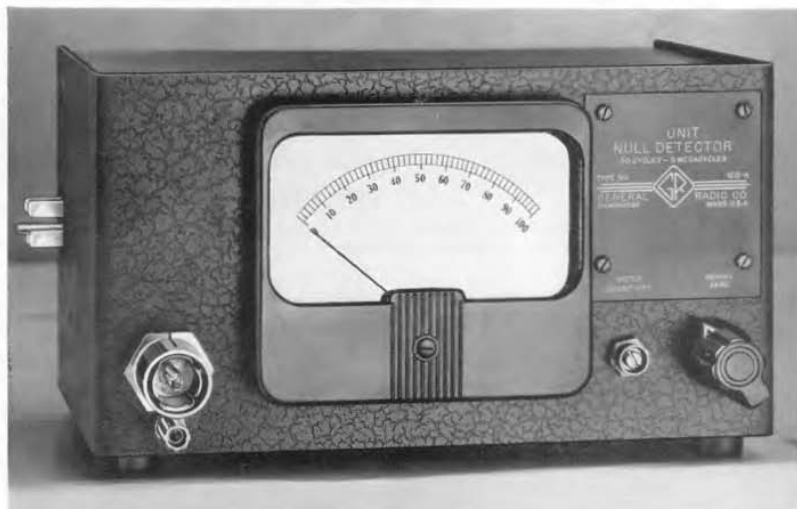
Figure 1. Panel view of the Unit Null Detector. The plug at the left connects to the Type 1203-A or Type 1204-B Unit Power Supply. At the option of the user, the power supply may be plugged in for easy assembly and disassembly or permanently bolted to the instrument to form a complete rigid assembly.
