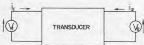
Figure 1. Functional diagram of a four-terminal transducer.
