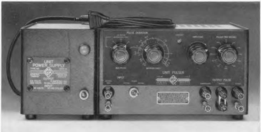
Figure 1. Panel view of the Type 1217-A Unit Pulser with the Type 1203-A Unit Power Supply.
