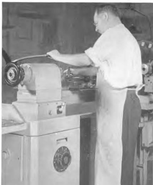
Figure 1. The new Type 1704-B Variac Speed Control installed on a bench lathe. The controller is installed just below the headstock where it is conveniently accessible, and the Variac, which is the speed adjustment control, is below the controller, on the bench cabinet. The chassis, which carries the transformers and rectifiers, is inside the cabinet.
