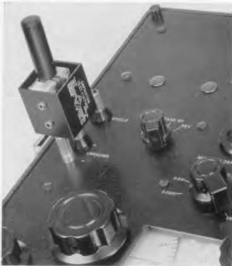
Figure 4. The fixture plugs easily fit into the terminals of General Radio bridges or into other equipment having jack-top binding posts, spaced 3/4 inch. The bridge shown here is a Type 1611-A Capacitance Test Bridge, and the capacitor is a tubular paper type.
