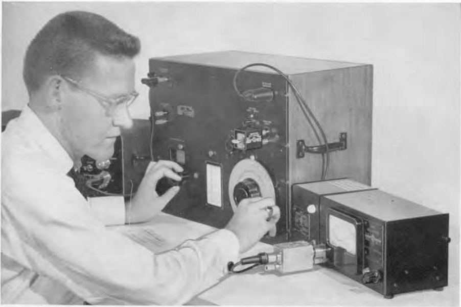
Figure 2. View of equipment for measuring disc-type capacitors at one megacycle. The Capacitor Test Fixture is installed on a Type 716-CS1 Capacitance Bridge. The generator is a Type 1330-A Oscillator, and the detector, a Type 1212-A Unit Null Detector. A one-megacycle filter is used at the input of the detector to reduce harmonics and noise.
