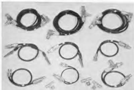
Figure 4. Connectors supplied with the Type P-579 Tester for connecting it to the many types of fuel gages now in use.
