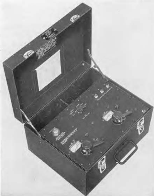
Figure 1. View of the Type P-579 Field Variable Capacitance Tester, mounted in its transit case.
