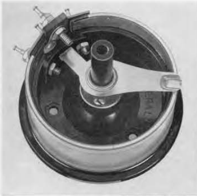
Figure 9. Type 314-S86 Variable Delay Line. Z_0 = 200 ohms, maximum time delay, 0.5 \mu\text{sec} (500 millimicroseconds).
