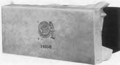
(2) Paper and wood-reinforced cardboard protect panel.
