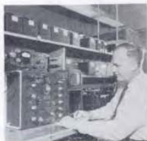
John F. Hersh, author of the article describing the new precision inductance bridge, is shown operating the bridge in the General Radio standards laboratory.
