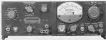
Panel view of the Bridge Oscillator-Detector Assembly.
