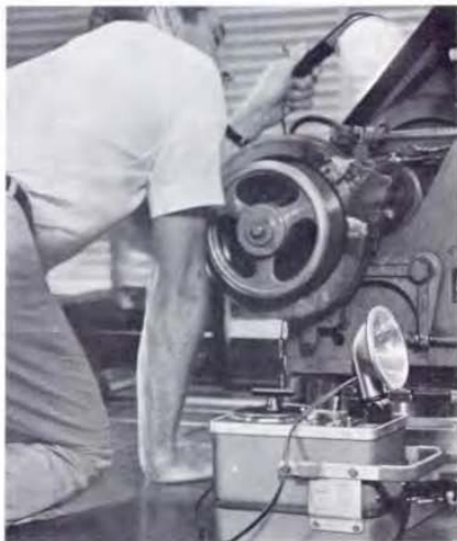
The extension lamp solves a logistics problem. Six-foot cord attaches through connector on front panel of Strobotac.
