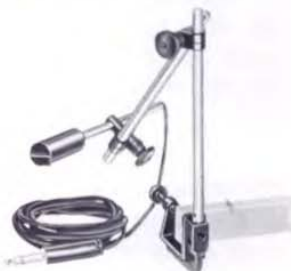
The Type 1537-A Photoelectric Pickoff is identical in appearance with the Type 1536-A. Only difference is that the Type 1536-A contains a light source, the Type 1537-A does not.
