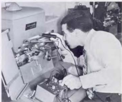
Using the Stroboslave as a diagnostic tool. The reflector has been slipped off so that the strobe lamp can probe the innards of the addressing machine. A photoelectric pickoff keeps the flashes synchronized with the machine, while a flash-delay unit allows the operator to scan the motion throughout its cycle.
