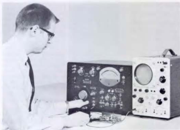
Figure 7. The Type 1309-A Oscillator and associated equipment used for testing of an audio amplifier.
