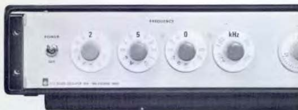
Figure 2. In-line readout of frequency with positioned decimal point and units. Least significant digit is continuously variable with a detent at zero.
