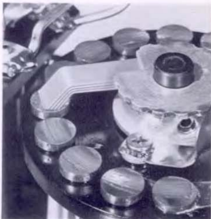
The use of multi-leaf wipers on silver-overlaid studs assures a contact resistance that varies by less than 100 microhms.
