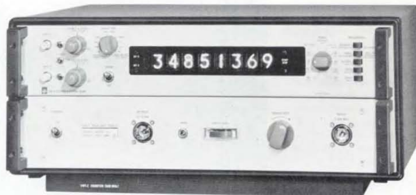
The 1191-Z Counter. The 500-MHz model is shown here in its bench version.
